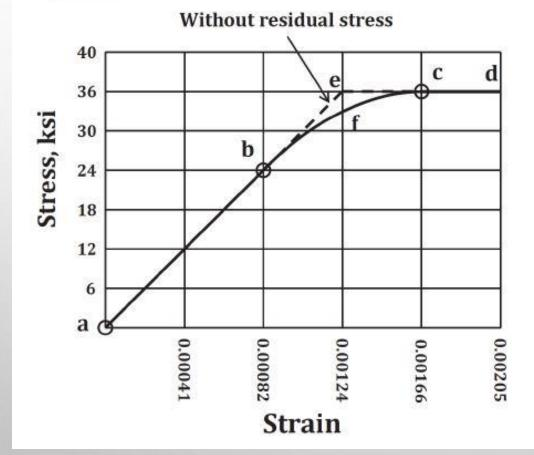
Due to presence of residual stress/strain the average stressstrain behavior follows path a-b-f-c-d
