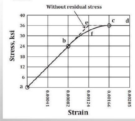
Due to presence of residual stress/strain the average stressstrain behavior follows path a-b-f-c-d
