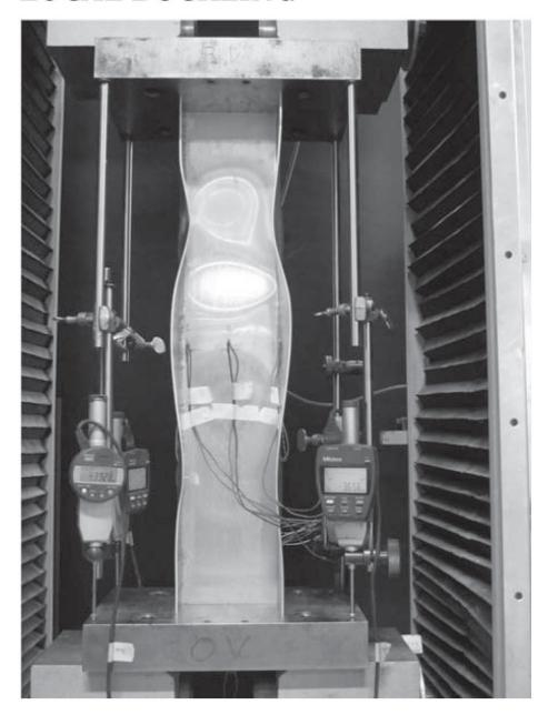
Local buckling primarily depends on the ratio, b/t, of the width (b) and thickness (t) of the plate elements that builds up a section.
