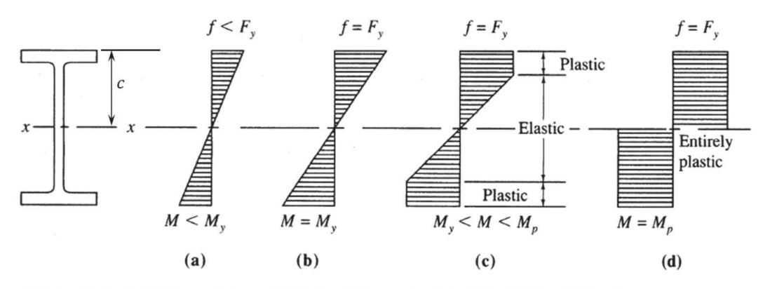
When the yield stress is reached at the extreme fiber [Fig. (b)], the nominal moment strength  $M_n$  is referred to as the yield moment  $M_y$  and is computed as
