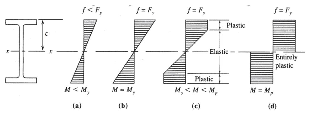
When the condition of Fig. (d) is reached, every fiber has a strain equal to or greater than  $\varepsilon_y = F_y/E_s$  i.e., it is in the plastic range. The nominal moment strength  $M_n$  is therefore referred to as the plastic moment  $M_p$ , and is computed as.
