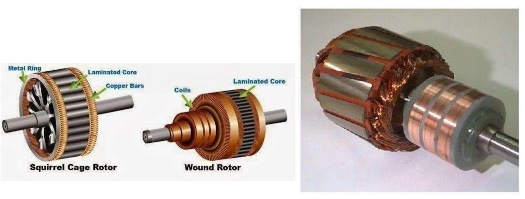
A wound rotor has a 3-phase winding, similar to the stator winding.
