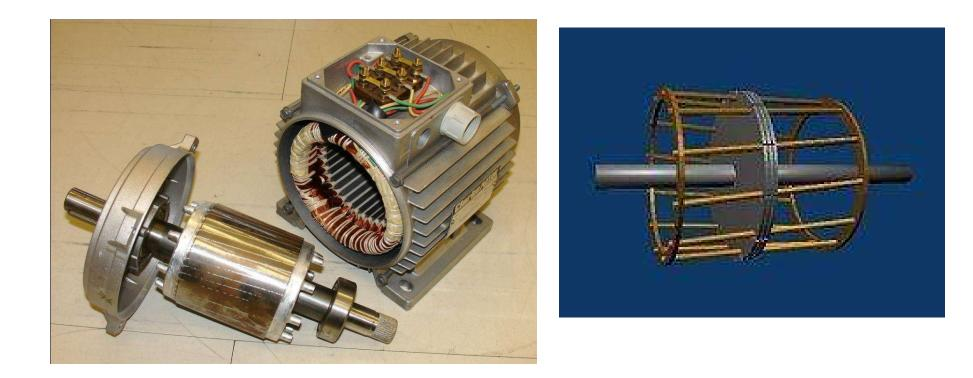
Squirrel cage rotor consists of copper bars, slightly longer than the rotor, which are pushed into the slots. The ends are welded to copper end rings, so that all the bars are short circuited. In small motors, the bars and end-rings are die cast in aluminum to form an integral block
