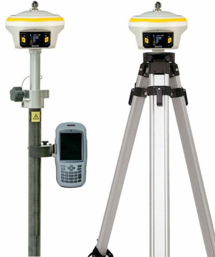
RTK GPS Base Station
