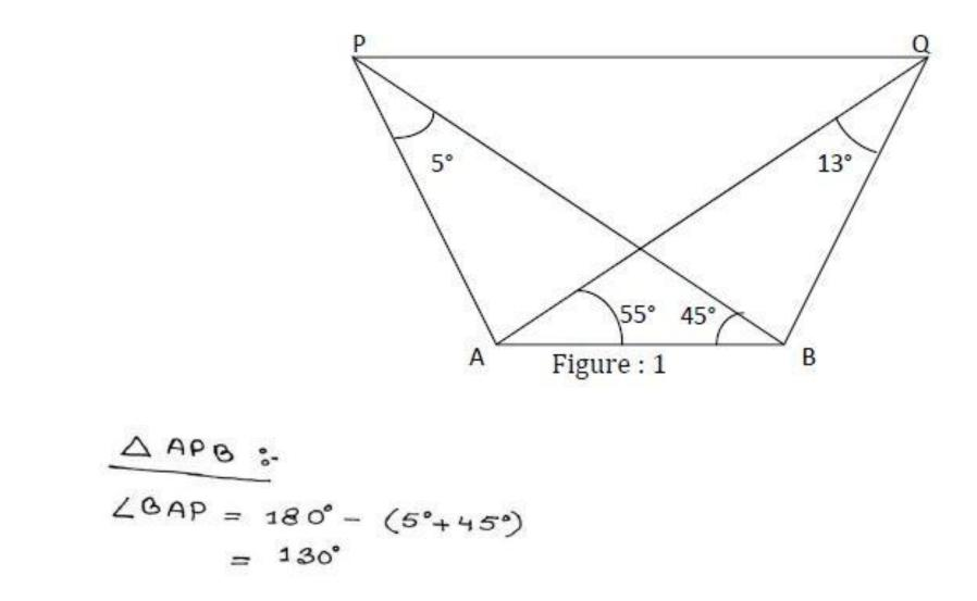
From DAPB.  $\frac{AP}{\sin LABP} = \frac{AB}{\sin LAPB}$  $\therefore AP = \frac{100'}{\sin 5^\circ} \times \sin 45^\circ$ = 811.31' From AABQ, AQ Sin LAGQ = AB Sin LAGB  $AQ = \frac{100'}{5in 13^{\circ}} * sin \{180^{\circ} - (55^{\circ} + 13^{\circ})\}$ = 100' \* Sin 112° Sin 13° = 412.17'
