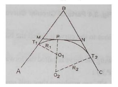
Reverse Curve: It consists of two circular arcs of same or different radii, having their centres to the different sides of the common tangent.
