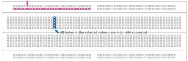
To interconnect the selected row (Node A) and column (node B) a cable going from any hole in the row to any hole in the column is needed:
