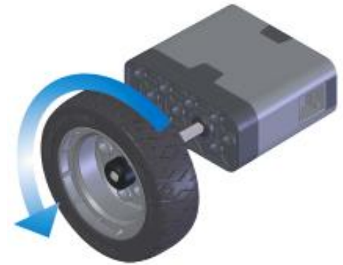
Motor applies torque to overcome the friction of a wheel turning against the ground
