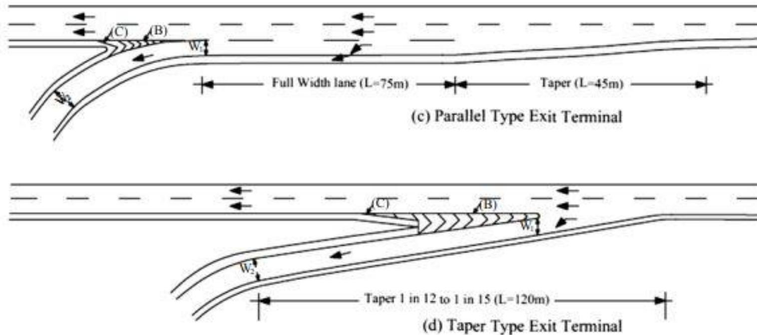
**Fig. 6.3 Typical Designs for Entry and Exit Terminals**
