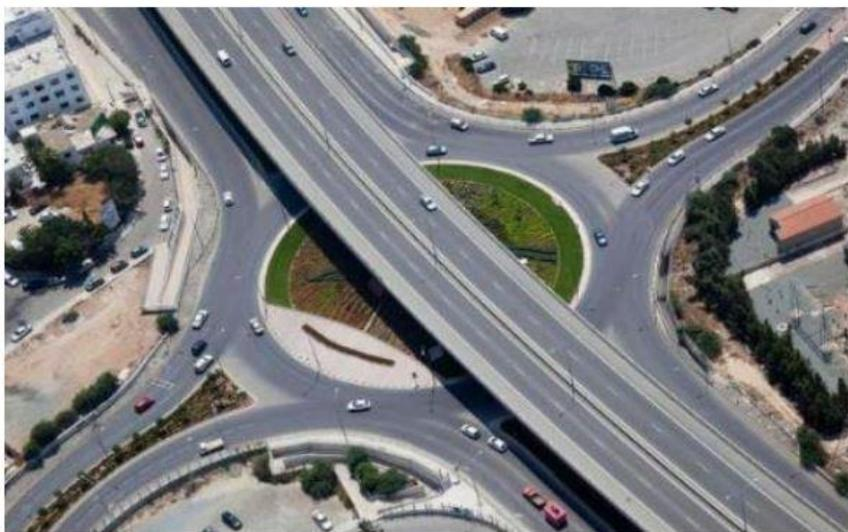
Figure 16 Three-Level Roundabout Interchange
