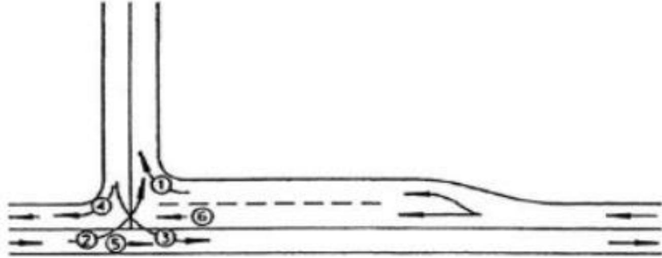
Figure 27 T-Intersection with Right-Turn Lane
