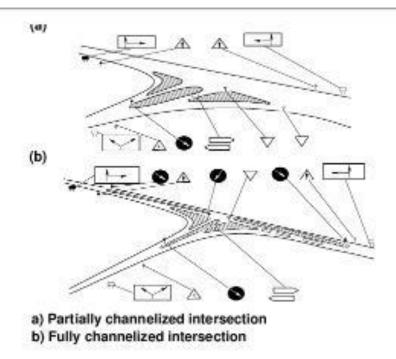
Figure 15: Channelized Intersection ensuring safety
