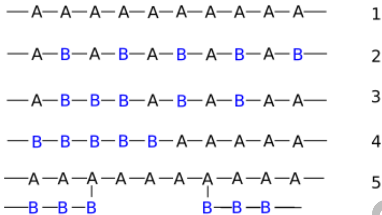
Figure 2. Different types of polymers: 1) homopolymer 2) alternating copolymer 3) random copolymer 4) block copolymer 5) graft copolymer.
