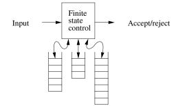
Figure 8.20: A machine with three stacks
