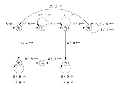
Figure 8.12: Transition diagram for the TM of Example 8.4
