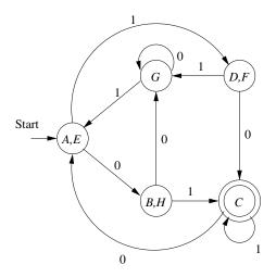
Figure 4.12: Minimum-state DFA equivalent to Fig. 4.8
