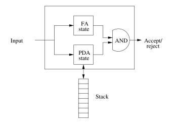
Figure 7.9: A PDA and a FA can run in parallel to create a new PDA
