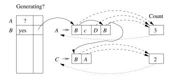
Figure 7.11: Data structure for the linear-time emptiness test
