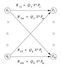
Figure 3.8: Result of eliminating state s from Fig. 3.7
