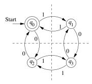
Figure 2.6: Transition diagram for the DFA of Example 2.4
