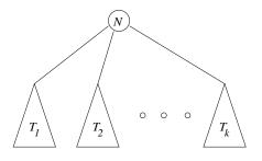
Figure 1.7: Inductive construction of a tree
