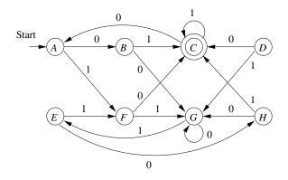
Figure 4.8: An automaton with equivalent states
