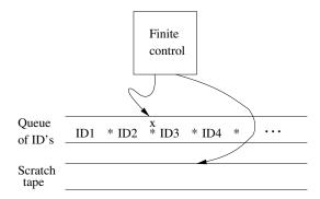
Figure 8.18: Simulation of an NTM by a DTM
