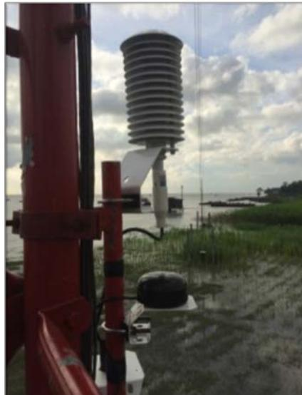
**Figure 16. Temperature sensor at Chandpur.**
