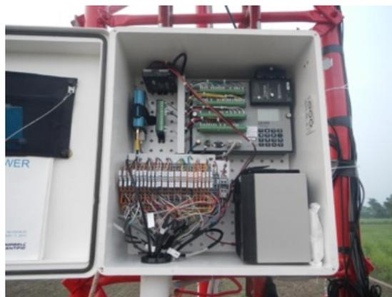
**Figure 19. Enclosure with data logger.**
