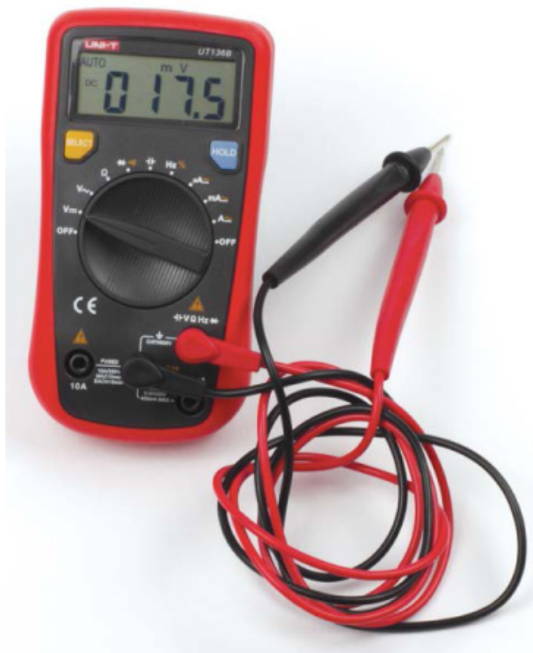
FIGURE 3-17 A multimeter, set to read voltage
