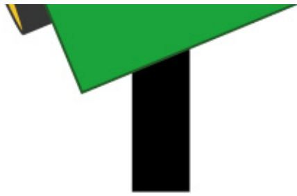
FIGURE 7-7 The robot turns left or right if one of the sensors detects the black line.
