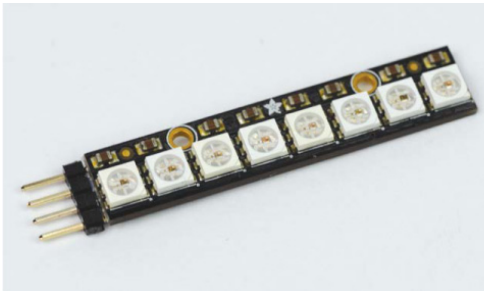
FIGURE 6-4 NeoPixel Stick with headers soldered on
