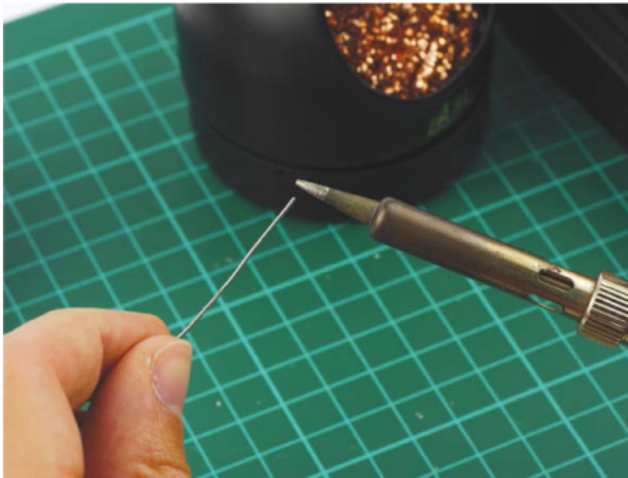
FIGURE D-6 Tinning the tip of my soldering iron
