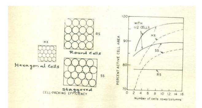
As an approximation it can be stated that: Size of the module  $\approx 15$  x diameter of the cell Half cells fill out end spaces when staggered pack is used. A slight gain in packing efficiency is obtained by utilizing half cells.
