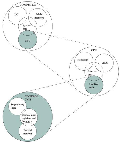
Figure 1.1 The Computer: Top-Level Structure
