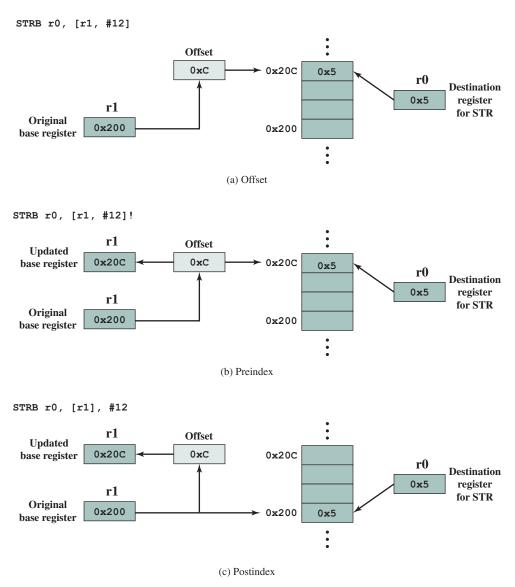
Figure 13.3 ARM Indexing Methods
