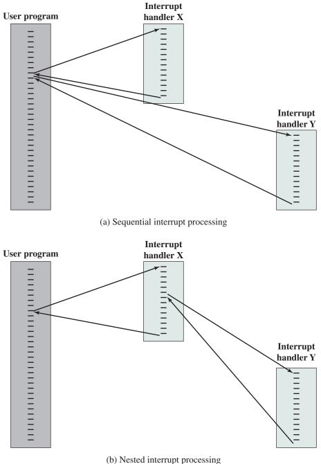
Figure 3.13 Transfer of Control with Multiple Interrupts
