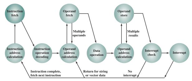
Figure 3.12 Instruction Cycle State Diagram, with Interrupts
