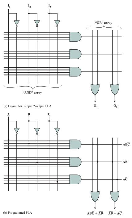
Figure 11.32 An Example of a Programmable Logic Array (PLA)
