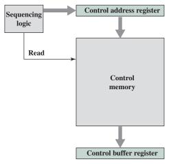
Figure 21.3 Control Unit Microarchitecture
