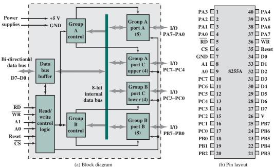
Figure 7.9 The Intel 8255A Programmable Peripheral Interface
