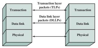
Figure 3.22 PCIe Protocol Layers
