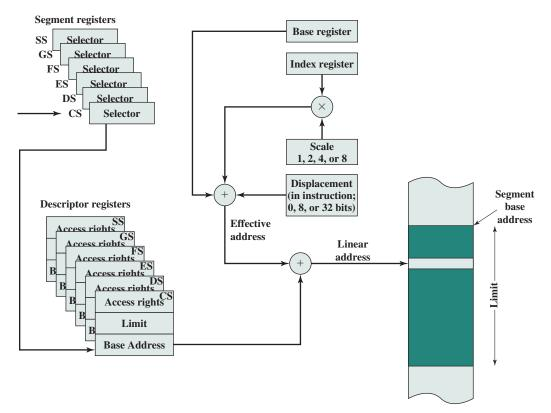
Figure 13.2 x86 Addressing Mode Calculation
