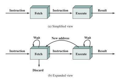
Figure 14.9 Two-Stage Instruction Pipeline
