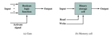
Figure 1.10 Fundamental Computer Elements
