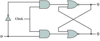
Figure 11.25 D Flip-Flop
