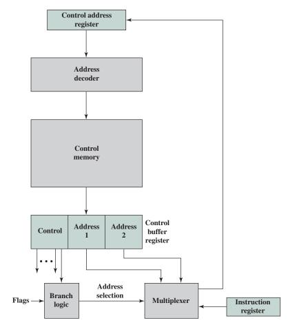
Figure 21.6 Branch Control Logic: Two Address Fields
