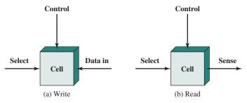
Figure 5.1 Memory Cell Operation
