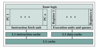
(b) Simultaneous multithreading
