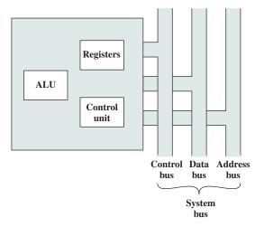
Figure 14.1 The CPU with the System Bus
