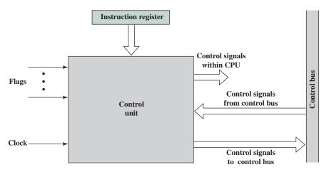
Figure 20.4 Block Diagram of the Control Unit
