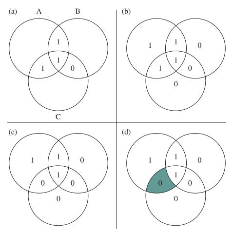
Figure 5.8 Hamming Error-Correcting Code
