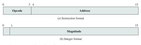
Program counter (PC) = Address of instruction Instruction register (IR) = Instruction being executed Accumulator (AC) = Temporary storage
