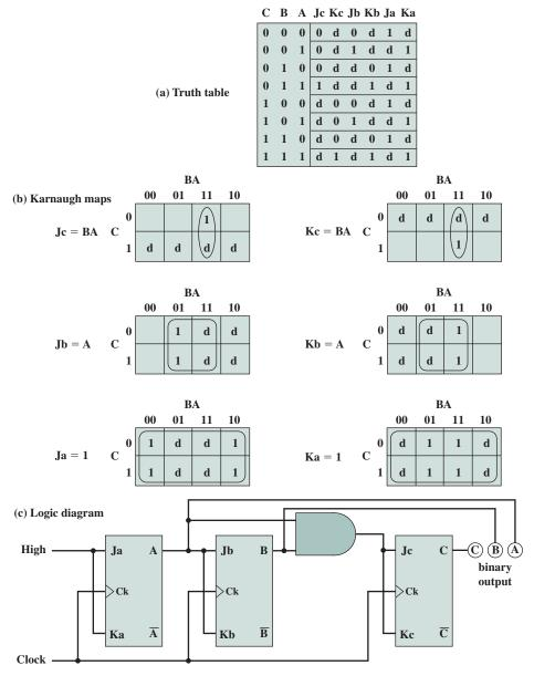
Figure 11.31 Design of a Synchronous Counter
