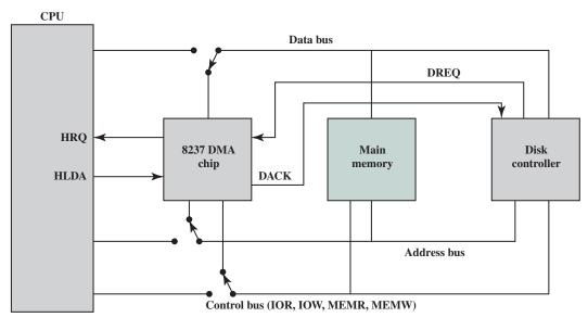
DACK = DMA acknowledge DREQ = DMA request HLDA = HOLD acknowledge HRQ = HOLD request
