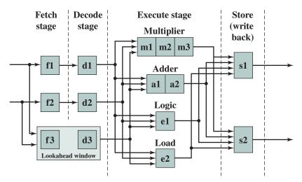
Figure 16.15 A Dual-Pipeline Superscalar Processor
