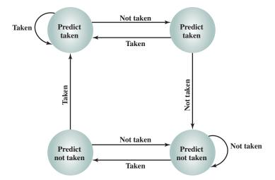
Figure 14.19 Branch Prediction State Diagram
