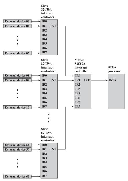
Figure 7.8 Use of the 82C59A Interrupt Controller
