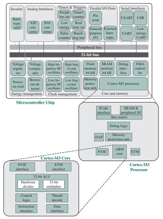
Figure 1.16 Typical Microcontroller Chip Based on Cortex-M3
