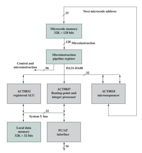
Figure 21.17 TI 8800 Block Diagram
