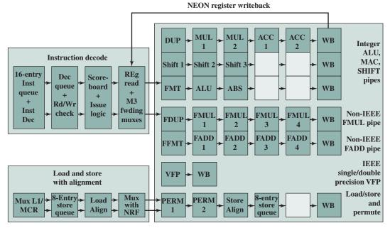
Figure 16.11 ARM Cortex-A8 NEON and Floating-Point Pipeline
