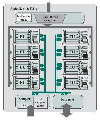
Figure 19.10 Intel Gen8 Subslice
