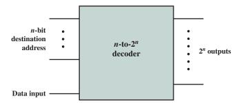
Figure 11.17 Implementation of a Demultiplexer Using a Decoder
