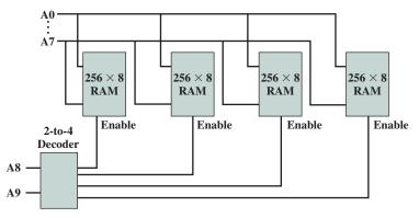
Figure 11.16 Address Decoding
