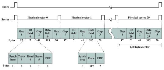
Figure 6.4 Winchester Disk Format (Seagate ST506)
