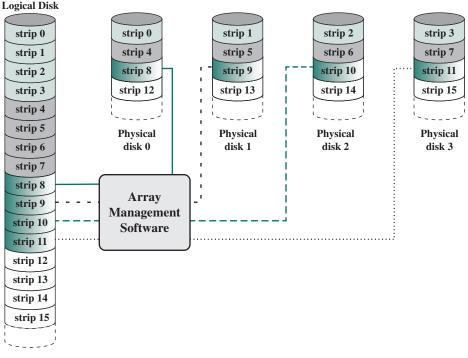
Figure 6.7 Data Mapping for a RAID Level 0 Array
