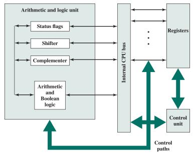
Figure 14.2 Internal Structure of the CPU
