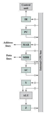
Figure 20.6 CPU with Internal Bus
