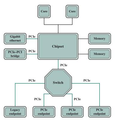
Figure 3.21 Typical Configuration Using PCIe
