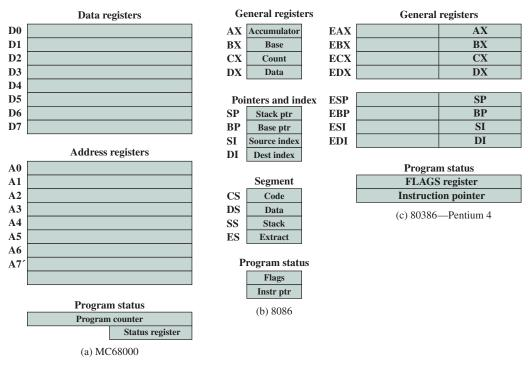
Figure 14.3 Example Microprocessor Register Organizations
