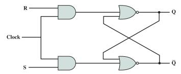
Figure 11.24 Clocked S–R Flip-Flop
