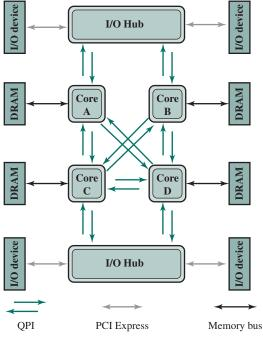
Figure 3.17 Multicore Configuration Using QPI
