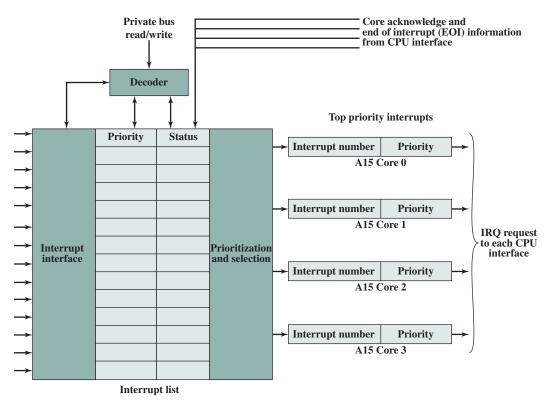
Figure 18.15 Generic Interrupt Controller Block Diagram
