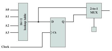
Figure 11.34 A Simple FPGA Logic Block
