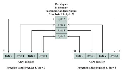
Figure 12.5 ARM Endian Support—Word Load/Store with E-Bit
