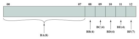
Figure 21.9 IBM 3033 Control Address Register
