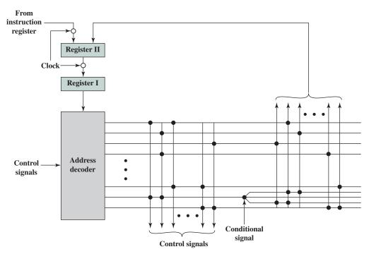
Figure 21.5 Wilkes's Microprogrammed Control Unit
