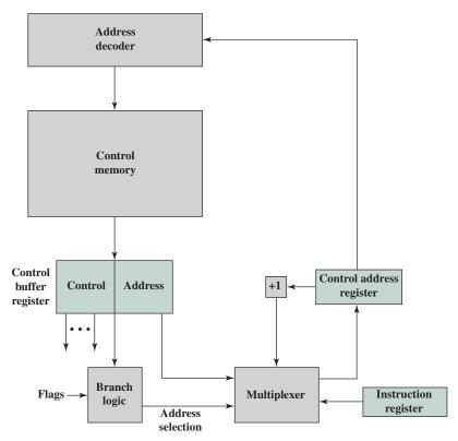
Figure 21.7 Branch Control Logic: Single Address Field
