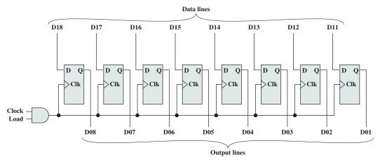
Figure 11.28 8-Bit Parallel Register
