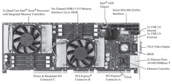
Figure 1.3 Motherboard with Two Intel Quad-Core Xeon Processors *Source:* Chassis Plans, www.chassis-plans.com
