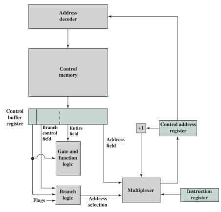
Figure 21.8 Branch Control Logic: Variable Format
