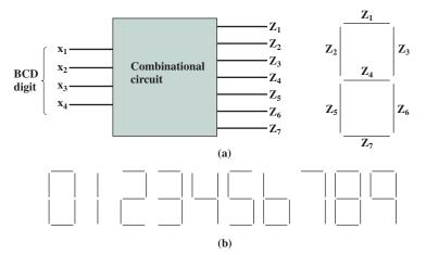
Figure 11.35 Seven-Segment LED Display Example
