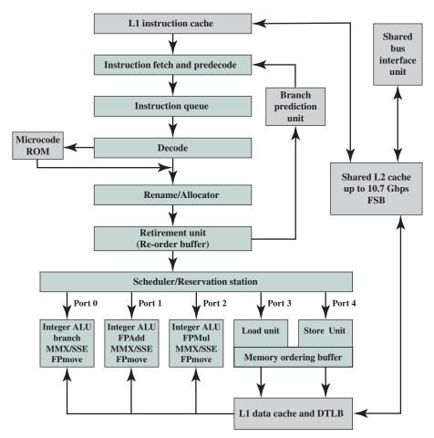
Figure 16.8 Intel Core Microarchitecture
