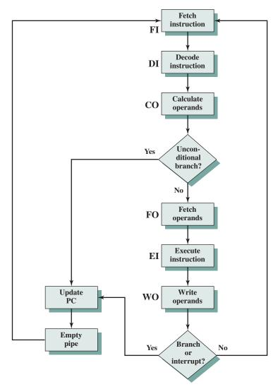
Figure 14.12 Six-Stage CPU Instruction Pipeline
