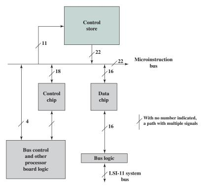
Figure 21.13 Simplified Block Diagram of the LSI-11 Processor
