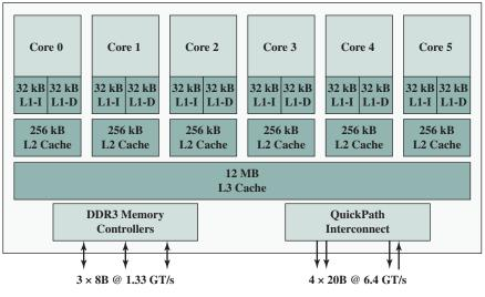
Figure 18.13 Intel Core i7-990X Block Diagram
