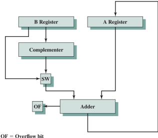
OF = Overnow bitSW = Switch (select addition or subtraction)
