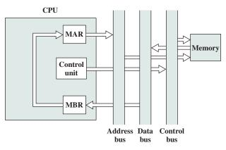
Figure 14.7 Data Flow, Indirect Cycle
