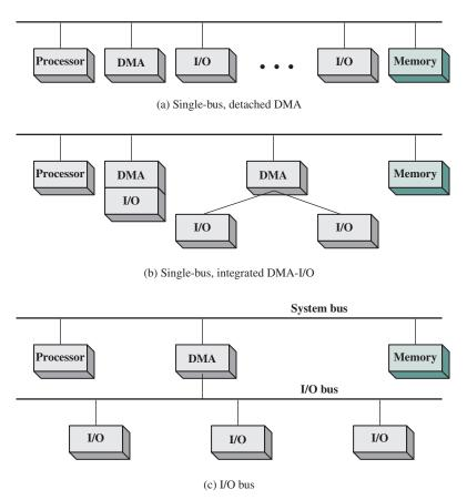
Figure 7.14 Alternative DMA Configurations
