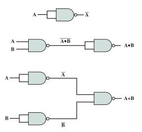
Figure 11.2 Some Uses of NAND Gates
