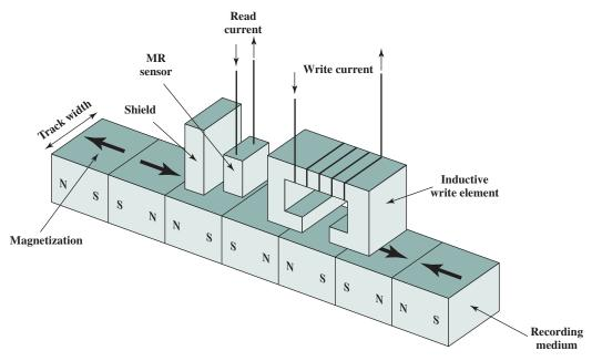
Figure 6.1 Inductive Write/Magnetoresistive Read Head
