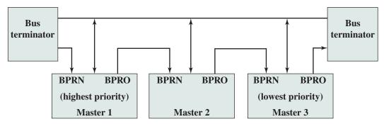
Figure 3.26 Multibus I Distributed Arbitration
