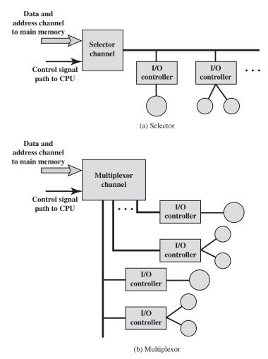
Figure 7.18I/O Channel Architecture
