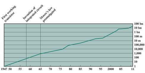
Figure 1.12 Growth in Transistor Count on Integrated Circuits
