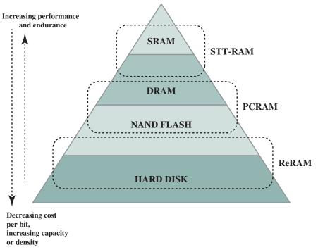
Figure 5.18 Nonvolatile RAM within the Memory Hierarchy
