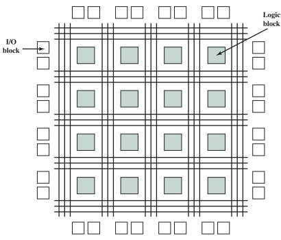
Figure 11.33 Structure of an FPGA
