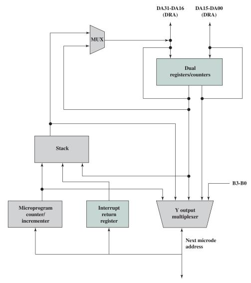
Figure 21.18 TI 8818 Microsequencer
