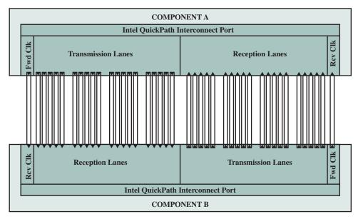
Figure 3.19 Physical Interface of the Intel QPI Interconnect
