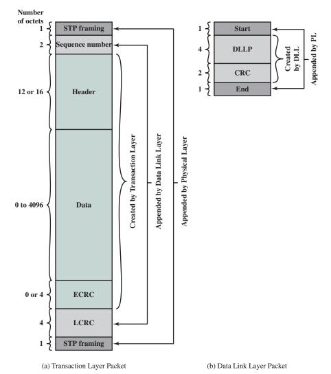
Figure 3.25 PCIe Protocol Data Unit Format
