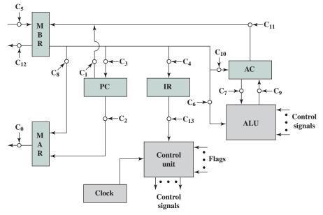
Figure 20.5 Data Paths and Control Signals
