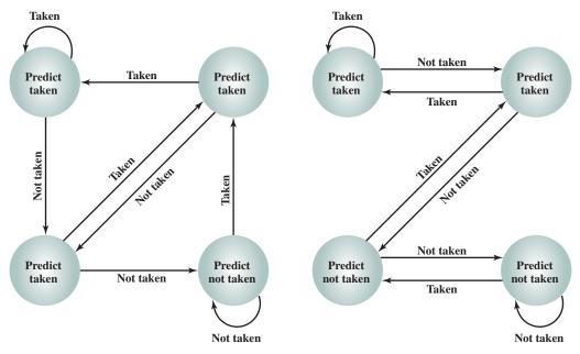
Figure 14.28 Two Branch Prediction State Diagrams
