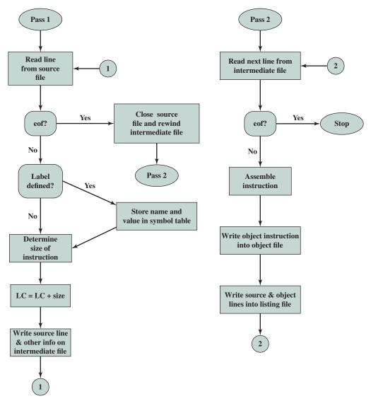
Figure B.4 Flowchart of Two-Pass Assembler
