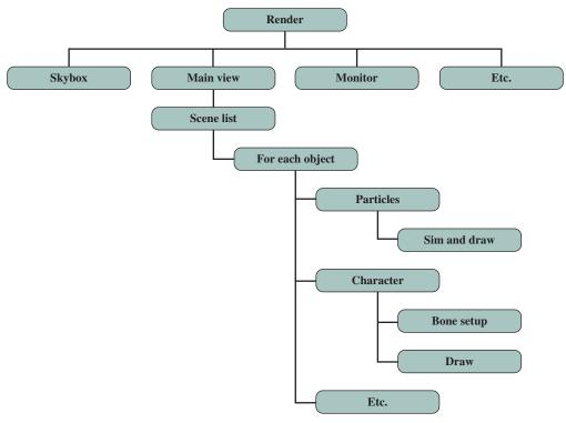
Figure 18.5 Hybrid Threading for Rendering Module
