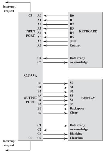
Figure 7.11 Keyboard/Display Interface to 8255A
