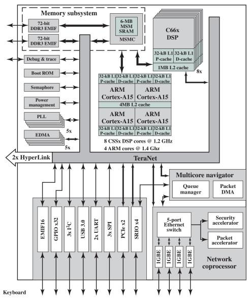
Figure 18.8 Texas Instruments 66AK2H12 Heterogenous Multicore Chip
