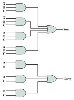
Figure 11.20 Implementation of an Adder
