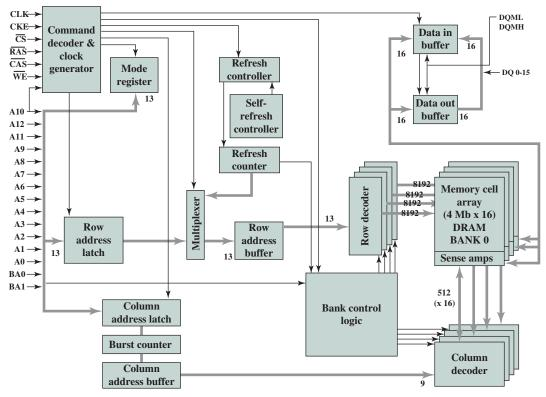
Figure 5.12 256-Mb Synchronous Dynamic RAM (SDRAM)
