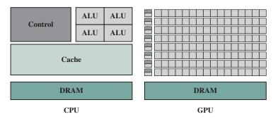
Figure 19.2 CPU versus GPU Silicon Area/Transistor Dedication
