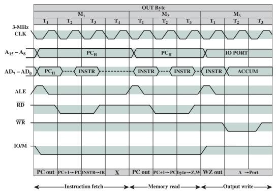
Figure 20.9 Timing Diagram for Intel 8085 OUT Instruction
