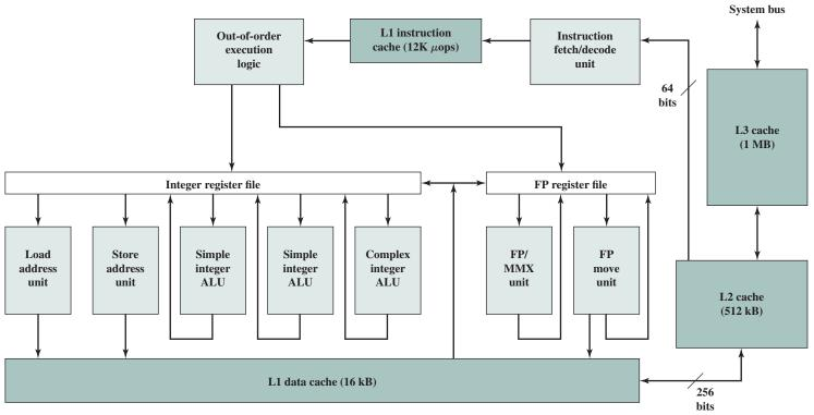
Figure 4.18 Pentium 4 Block Diagram
