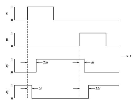
Figure 11.23 NOR S–R Latch Timing Diagram
