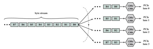
Figure 3.23 PCIe Multilane Distribution
