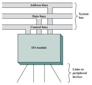
Figure 7.1 Generic Model of an I/O Module
