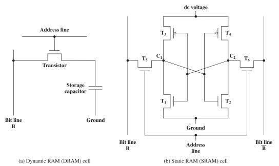
Figure 5.2 Typical Memory Cell Structures
