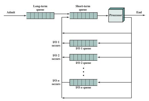
Figure 8.11 Queuing Diagram Representation of Processor Scheduling
