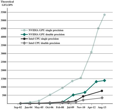
Figure 19.3 Floating-Point Operations per Second for CPU and GPU
