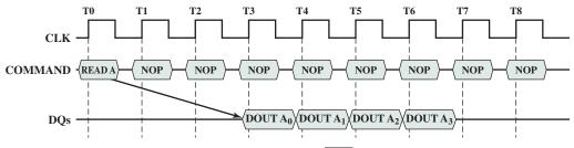
**Figure 5.13** SDRAM Read Timing (burst length =  $4, \overline{CAS}$  latency = 2)
