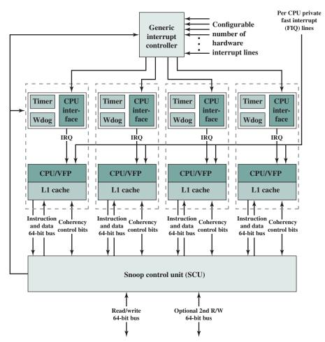
Figure 18.14 ARM Cortex-A15 MPCore Chip Block Diagram
