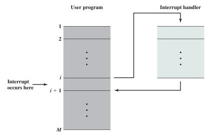
Figure 3.8 Transfer of Control via Interrupts
