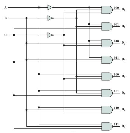
**Figure 11.15** Decoder with 3 Inputs and  $2^3 = 8$  Outputs
