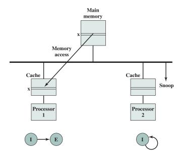
Figure 17.16 MESI Example: Processor 1 Reads Line x
