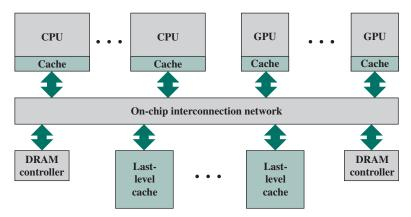
Figure 18.7 Heterogenous Multicore Chip Elements
