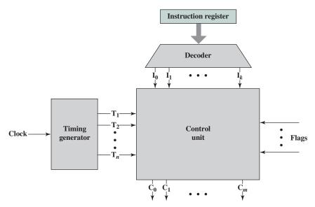
Figure 20.10 Control Unit with Decoded Inputs
