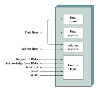
Figure 7.12 Typical DMA Block Diagram
