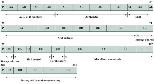
Figure 21.16 IBM 3033 Microinstruction Format
