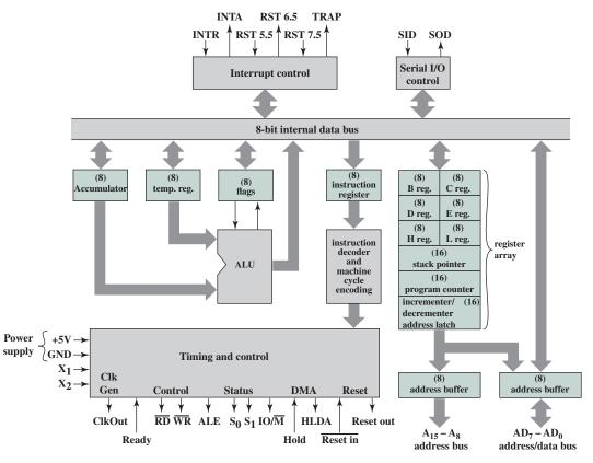
Figure 20.7 Intel 8085 CPU Block Diagram
