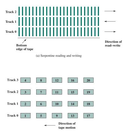
(b) Block layout for system that reads–writes four tracks simultaneously
