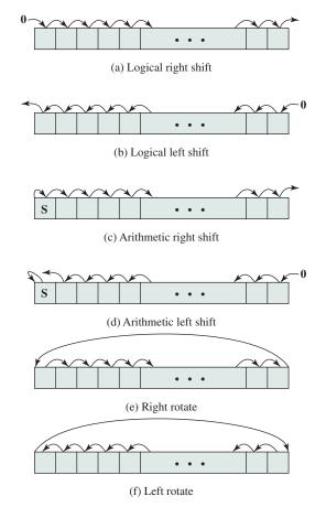
Figure 12.6 Shift and Rotate Operations
