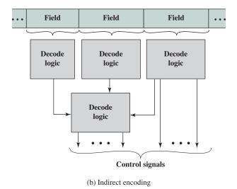
Figure 21.11 Microinstruction Encoding
