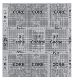
**Figure 1.4** zEnterprise EC12 Processor Unit (PU) chip diagram *Source:* IBM zEnterprise EC12 Technical Guide, December 2013, SG24-8049-01. IBM, Reprinted by Permission
