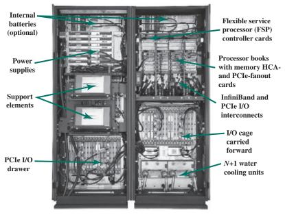
Figure 7.20 IBM zEC12 I/O Frames–Front View
