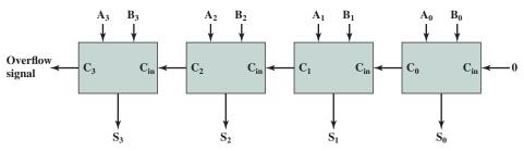
Figure 11.19 4-Bit Adder
