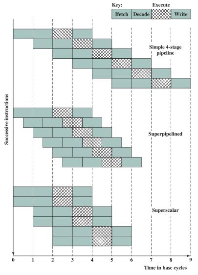
Figure 16.2 Comparison of Superscalar and Superpipeline Approaches
