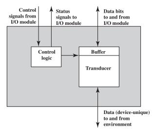
Figure 7.2 Block Diagram of an External Device
