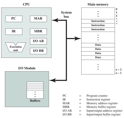
Figure 3.2 Computer Components: Top-Level View
