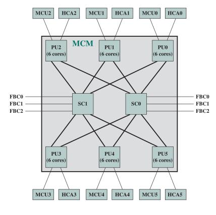
FBC = fabric book connectivityMCU = memory control unitHCA = host channel adapterPU = processor unitMCM = multichip moduleSC = storage control
