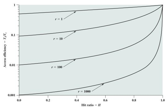
**Figure 4.22** Access Efficiency as a Function of Hit Ratio  $(r = T_2/T_1)$
