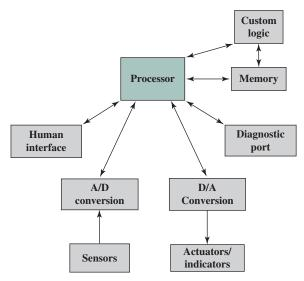
Figure 1.14 Possible Organization of an Embedded System
