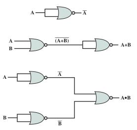
Figure 11.3 Some Uses of NOR Gates
