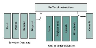
Figure 16.5 Organization for Out-of-Order Issue with Out-of-Order Completion
