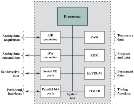
Figure 1.15 Typical Microcontroller Chip Elements
