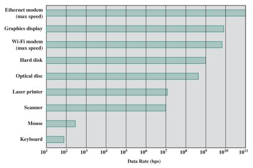
Figure 2.1 Typical I/O Device Data Rates
