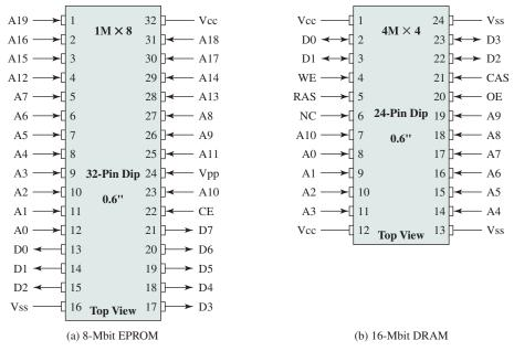
Figure 5.4 Typical Memory Package Pins and Signals
