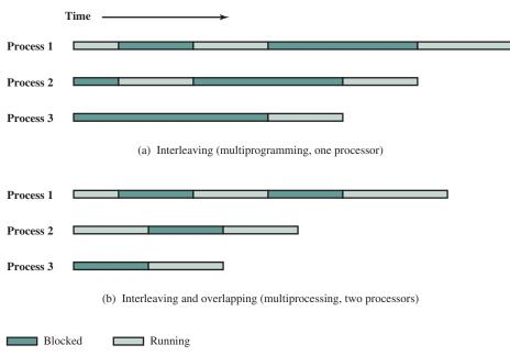
Figure 17.3 Multiprogramming and Multiprocessing
