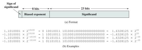
Figure 10.18 Typical 32-Bit Floating-Point Format
