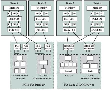
Figure 7.21 IBM zEC12 I/O System Structure
