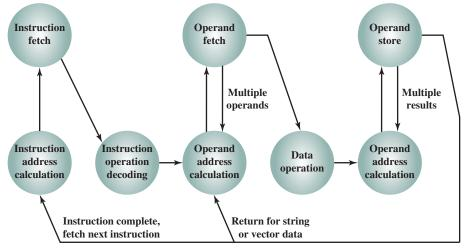
Figure 3.6 Instruction Cycle State Diagram
