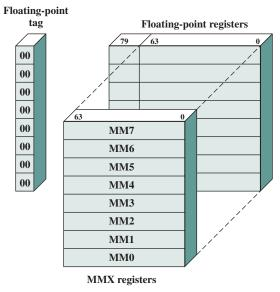
Figure 14.24 Mapping of MMX Registers to Floating-Point Registers
