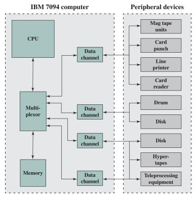
Figure 1.9 An IBM 7094 Configuration
