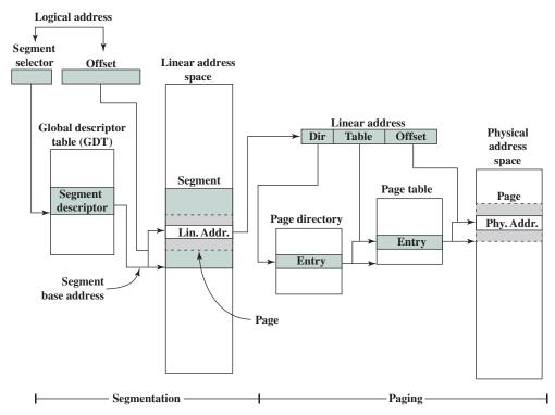
Figure 8.21 Intel x86 Memory Address Translation Mechanisms
