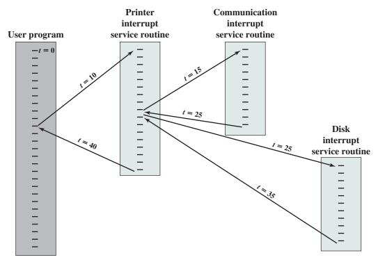
Figure 3.14 Example Time Sequence of Multiple Interrupts
