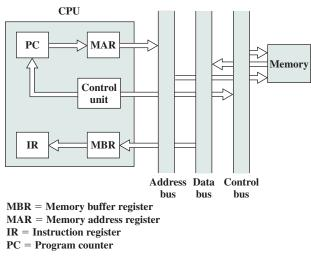
Figure 14.6 Data Flow, Fetch Cycle
