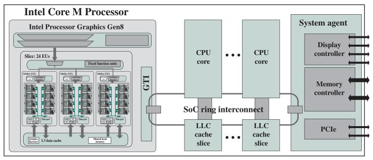
Figure 19.12 Intel Core M Processor SoC
