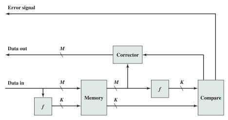
Figure 5.7 Error-Correcting Code Function
