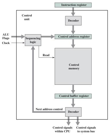
Figure 21.4 Functioning of Microprogrammed Control Unit
