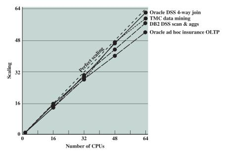
Figure 18.4 Scaling of Database Workloads on Multiple-Processor Hardware
