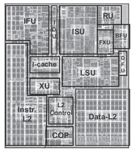
Figure 1.5 zEnterprise EC12 Core layout Source: IBM zEnterprise EC12 Technical Guide, December 2013, SG24-8049-01. IBM, Reprinted by Permission
