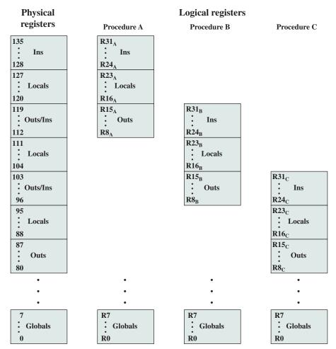
Figure 15.12 SPARC Register Window Layout with Three Procedures
