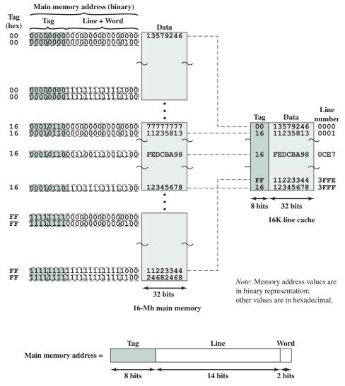
Figure 4.10 Direct Mapping Example
