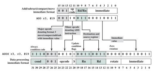
Figure 13.12 Expanding a Thumb ADD Instruction into its ARM Equivalent
