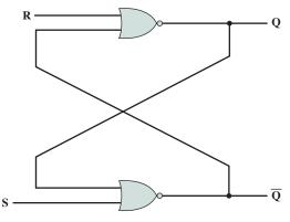
Figure 11.22 The S–R Latch Implemented with NOR Gates
