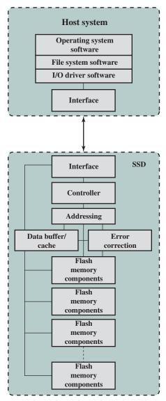
Figure 6.8 Solid State Drive Architecture
