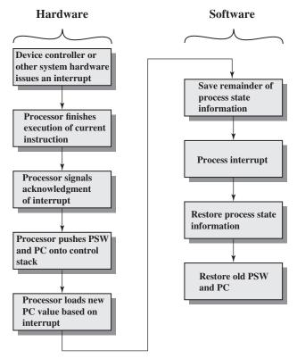
Figure 7.6 Simple Interrupt Processing
