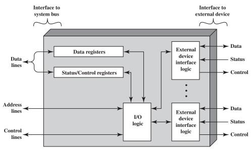
Figure 7.3 Block Diagram of an I/O Module
