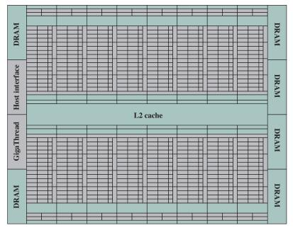
Figure 19.4 NVIDIA Fermi Architecture
