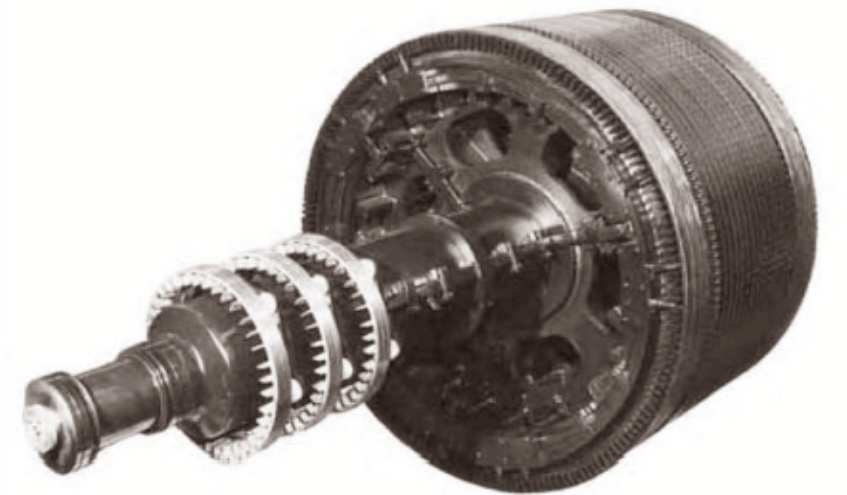
FIGURE 7-4 Typical wound rotors for induction motors. Notice the slip rings and the bars connecting the rotor windings to the slip rings. (Courtesy of General Electric Company.)
