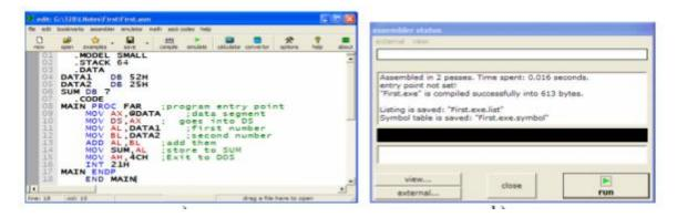
The compile button on the taskbar starts assembling and linking of the source file. A report window is opened after the assembling process is completed. Figure below shows the emulator of 8086 which gets opened by clicking on emulate button.
