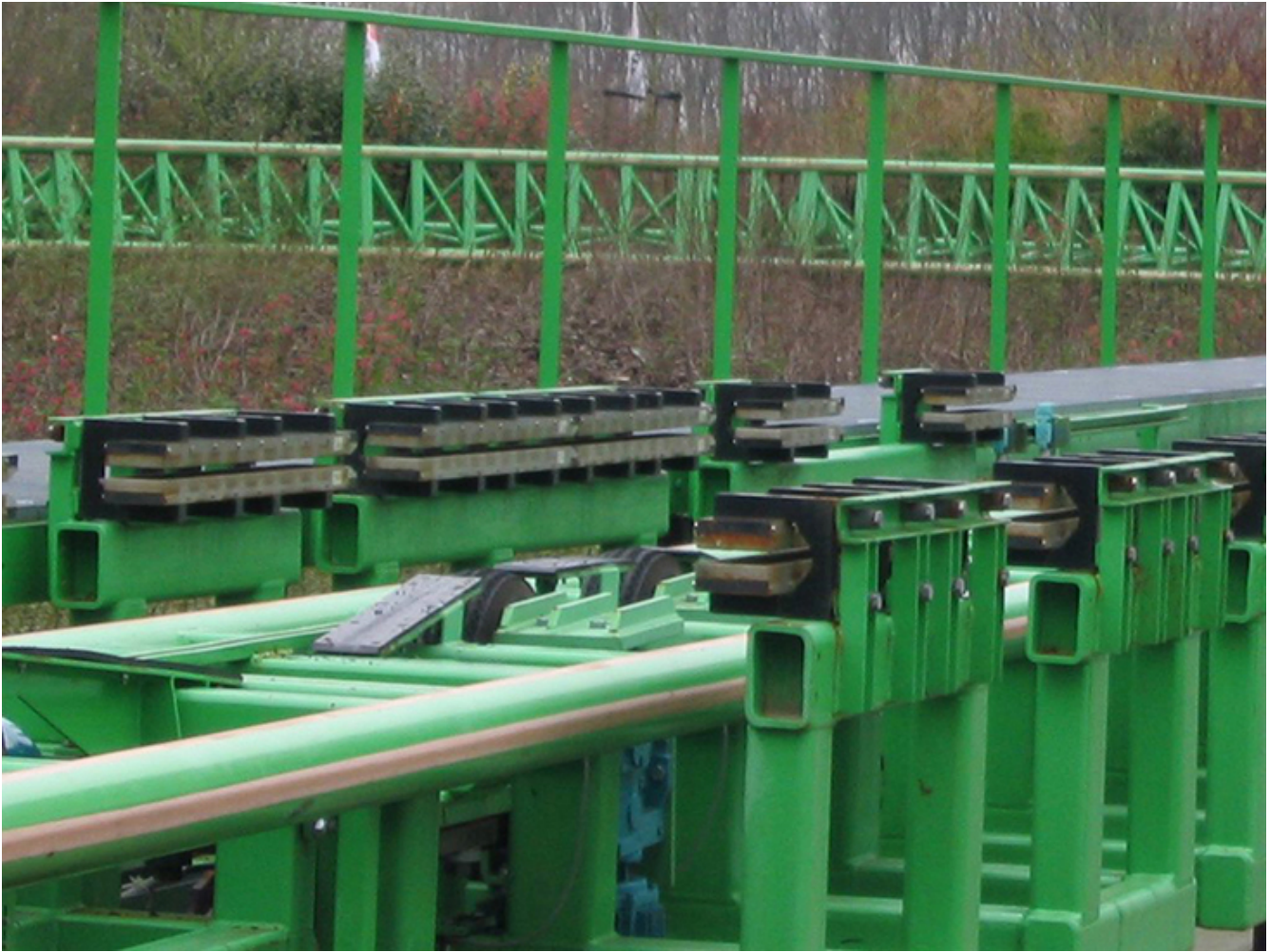
Figure 10.5.7 The rows of rare-earth magnets (protruding horizontally) are used for magnetic braking in roller coasters. (credit: Stefan Scheer)
