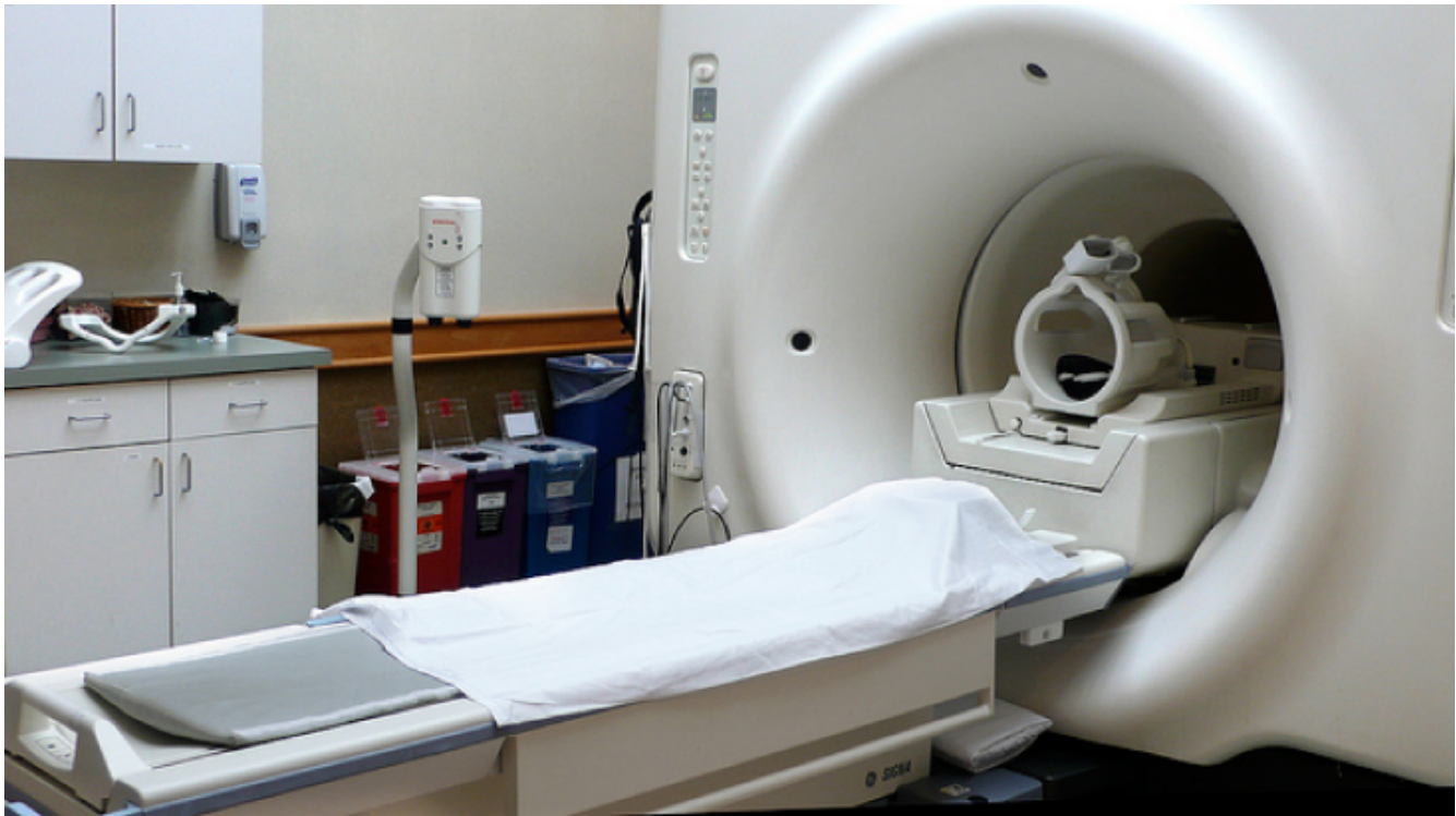
Figure 9.6.3 In an MRI machine, a large magnetic field is generated by the cylindrical solenoid surrounding the patient. (credit: Liz West)
