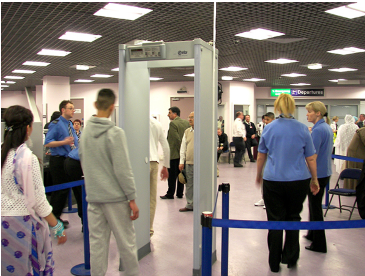
Figure 11.2.5 The familiar security gate at an airport not only detects metals, but can also indicate their approximate height above the floor. (credit: “Alexbuirds”/Wikimedia Commons)
