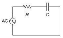
Equation number (2) represents the variation of current with time and shows that current leads the applied voltage in phase by an angle
