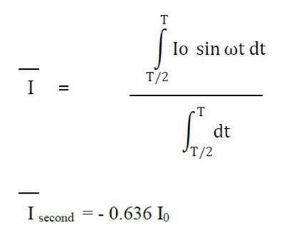
The average value of alternating current (Voltage) during the 1st and 2nd half cycles are equal but opposite in sign. i.e. they are alternatively positive and negative.
