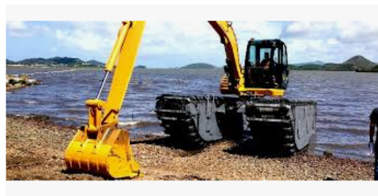
AMPHIBIOUS EXCAVATOR: swamp buggy ... gruasyparejos.com
