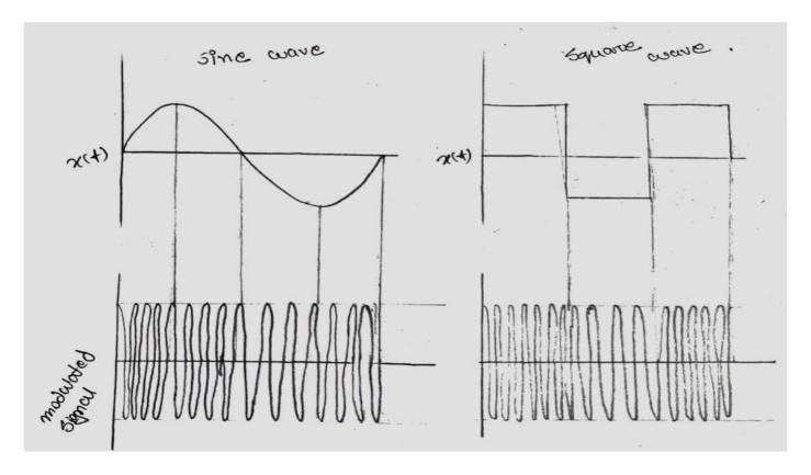
5. Find the FM modulation index if modulating signal is 100Cos(2\*pi\*1000\*t) and deviation constant is 20 Hz/volt.
