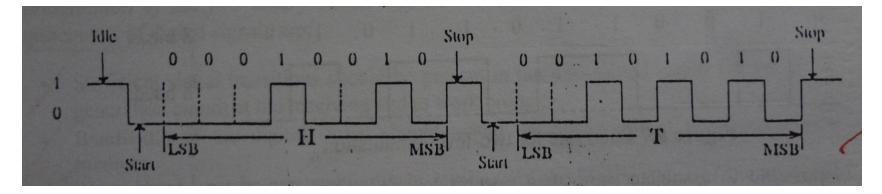
**Example problem 2:** Sketch the logic levels for the message 'HT' when it is transmitted in asynchronous mode with stop bit equal to one bit. Use ASCII code with **even** parity.
