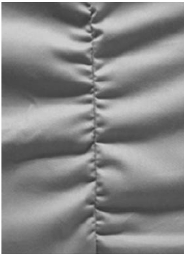
16.8 Pucker due to structural jamming.
