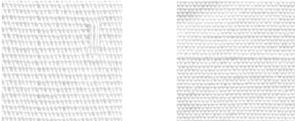
Figure 4.28: Warp-float and coarse-pick
