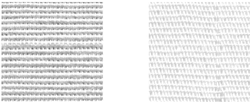
Figure 4.27: Double-pick and double-end
