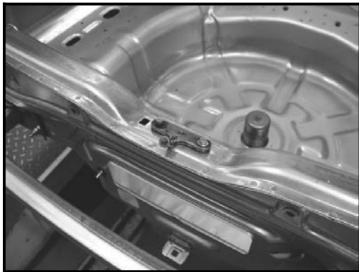
Fig. 3. The distance plate of the posterior boot door for the measurements of margins and external profiles
