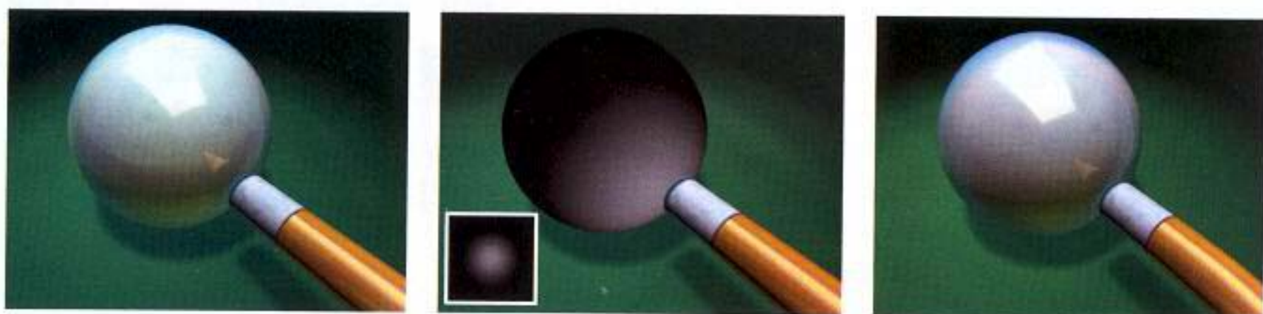
6.6 Notice the difference that the reflection map, middle, has made to the image on the right. It provides a more realistic portrayal of a pool ball's reflective quality than the image on the left.
