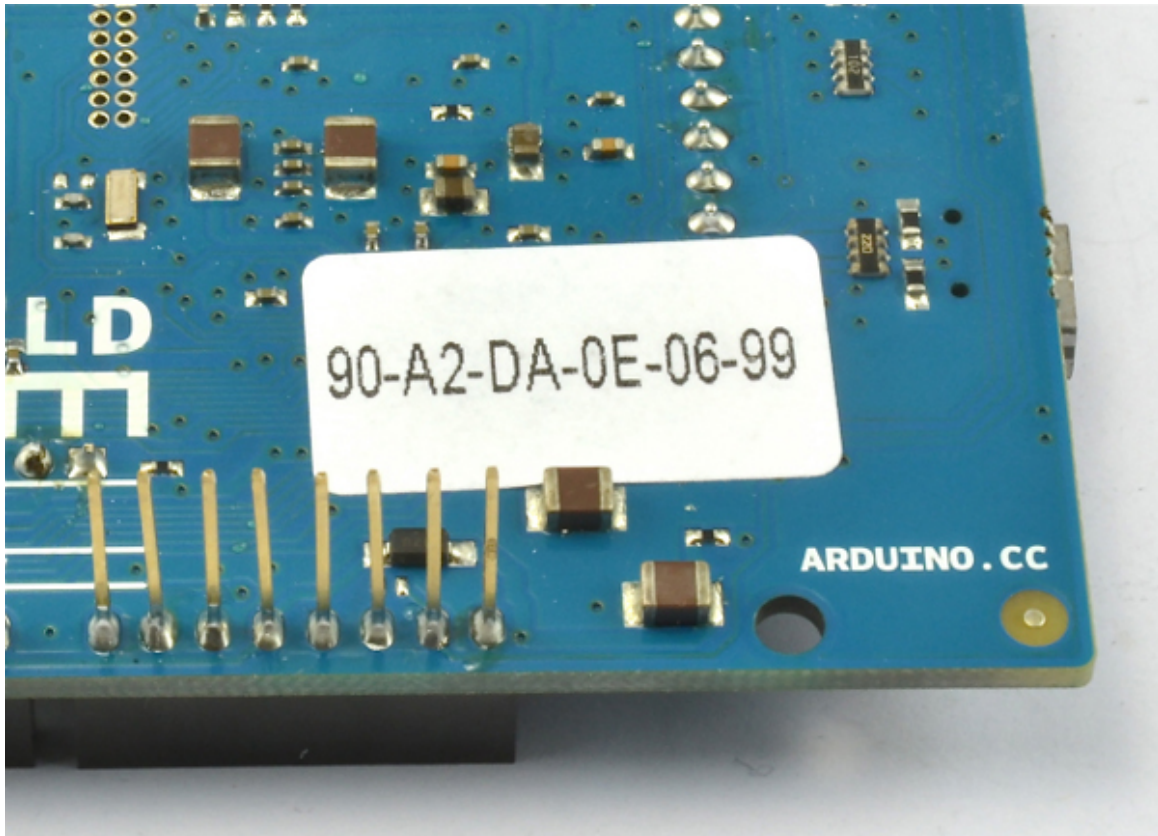
Figure 12-4 Mac address sticker on a WiFi Shield
