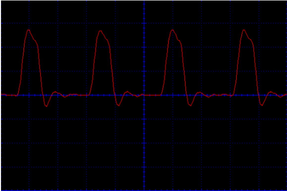
Figure 4-5 Generating a 4-MHz signal with an Arduino
