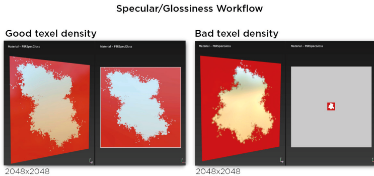
Figure 43: Providing a good texel density for UVs is the best method for minimizing any edge artifacts
