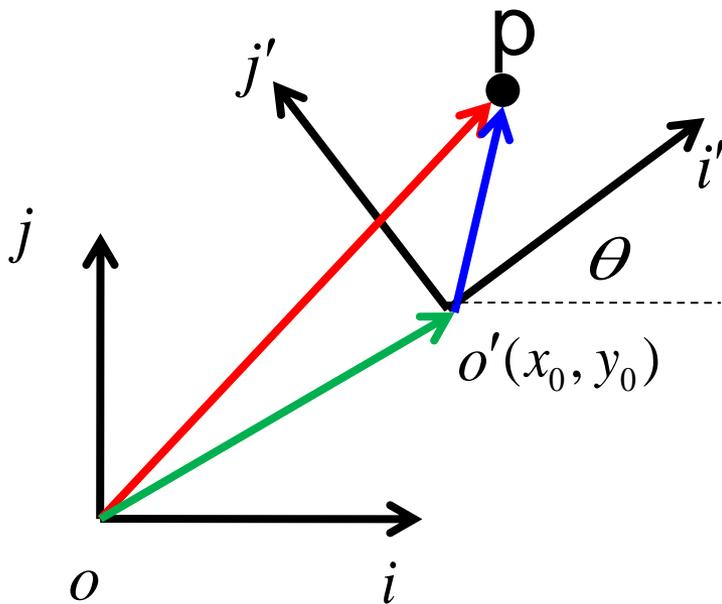
$$\begin{pmatrix} x \\ y \\ 1 \end{pmatrix} = \begin{pmatrix} \cos \theta & -\sin \theta & x_0 \\ \sin \theta & \cos \theta & y_0 \\ 0 & 0 & 1 \end{pmatrix} \begin{pmatrix} x' \\ y' \\ 1 \end{pmatrix}$$
