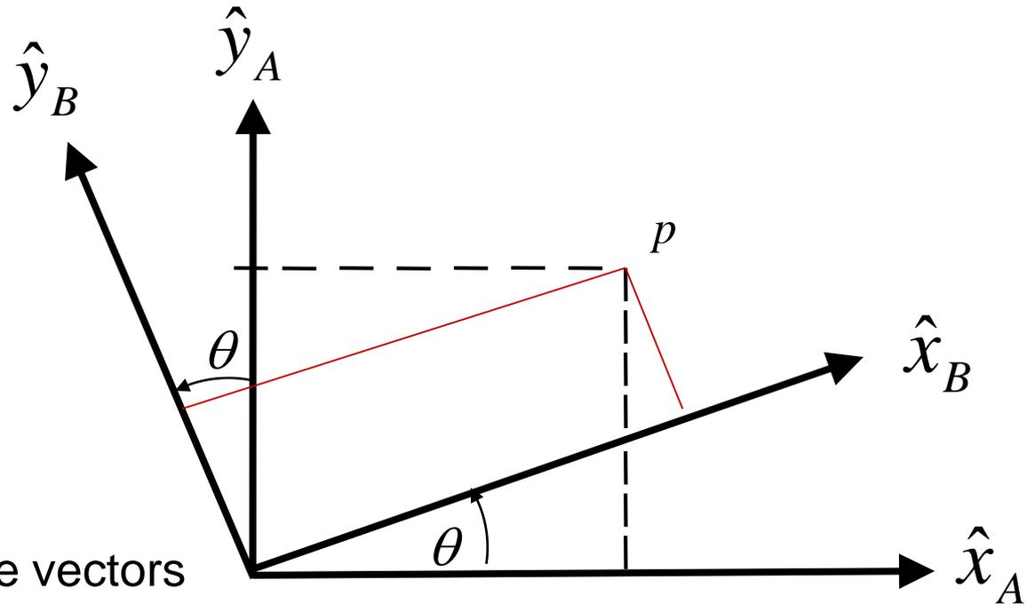
$\theta$ : The angle between  $\hat{x}_A$  and  $\hat{x}_B$  in anti clockwise direction
