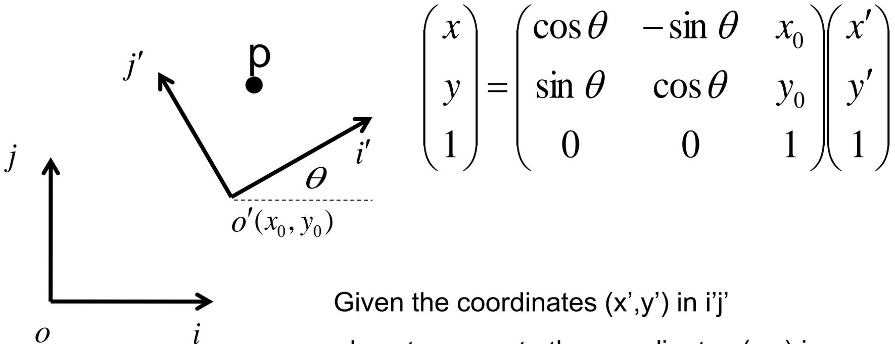
$$\begin{pmatrix} x \\ y \\ 1 \end{pmatrix} = \begin{pmatrix} \cos \theta & -\sin \theta & x_0 \\ \sin \theta & \cos \theta & y_0 \\ 0 & 0 & 1 \end{pmatrix} \begin{pmatrix} x' \\ y' \\ 1 \end{pmatrix}$$
