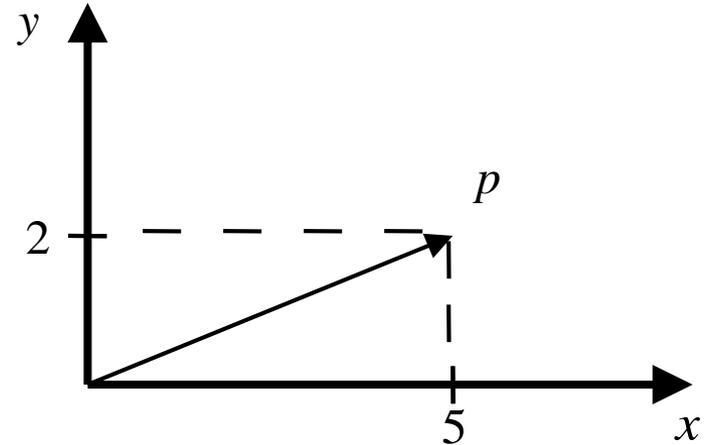
$\hat{x}$  ← A vector of length one pointing in the direction of the base frame x axis
