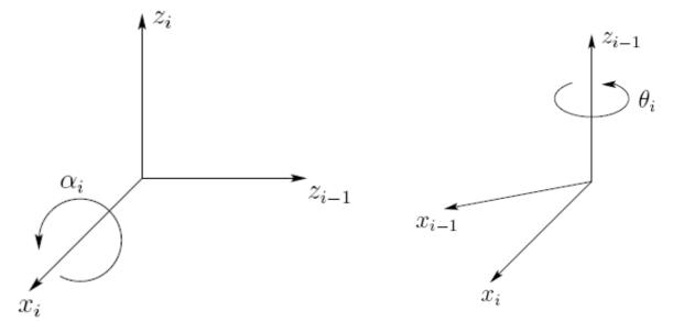
•Link twist  $\alpha_i$  :the angle from the  $Z_{i-1}$  axis to the  $Z_i$  axis about the  $X_i$  axis. The positive sense for  $\alpha$  is determined from  $z_{i-1}$  and  $z_i$  by the right-hand rule.
