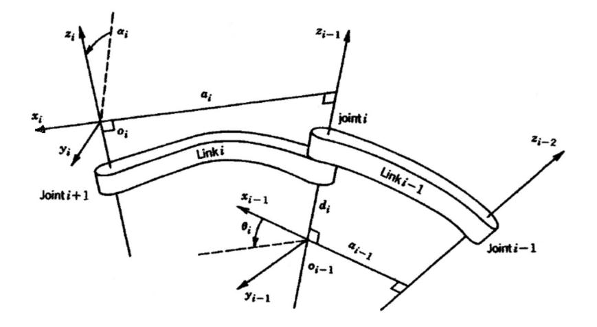
Step 1: Locate and label the joint axes  $z_0, \ldots, z_{n-1}$ .
