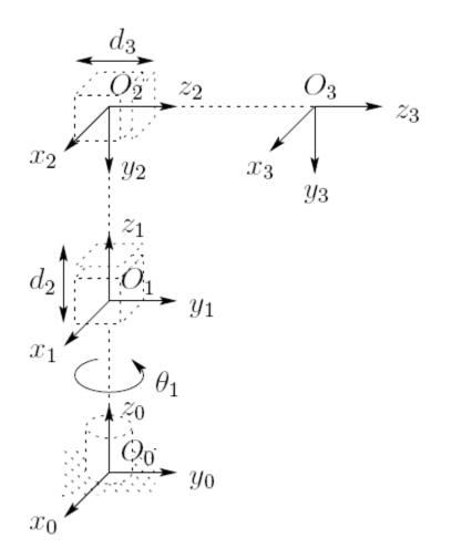
$$A_{1} = \begin{bmatrix} c_{1} & -s_{1} & 0 & 0 \\ s_{1} & c_{1} & 0 & 0 \\ 0 & 0 & 1 & d_{1} \\ 0 & 0 & 0 & 1 \end{bmatrix}$$
