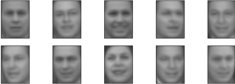
Figure 3-43. Cluster centers found by k -means when setting the number of clusters to 10
