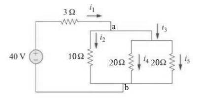
**Q4.** Using Nodal Analysis, find the node voltages and also the voltage  $v_o$ , Vab and Vcd.
