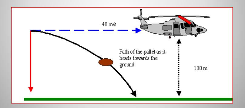
a) What is the horizontal velocity? B) Can you show that the vertical velocity is 44.7 m/s towards the ground? Note that the horizontal velocity is ignored, c) What is the resultant velocity of the pallet just before it hits the ground?
