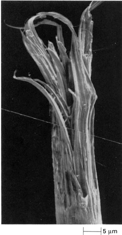
19.17 Fibrillar break of wet mercerised cotton.
