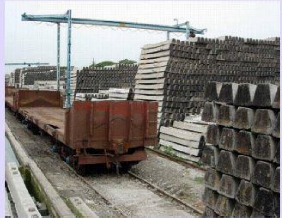
(n) Storage and dispatching of sleepers
