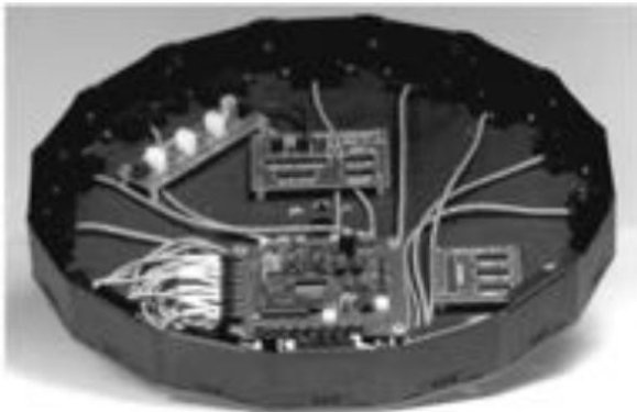
ring with 16 IR sensors
