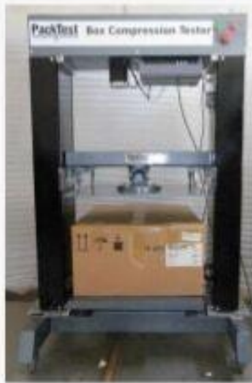
Mechanical Model (Runs with Motor driven Ball-Screw)
