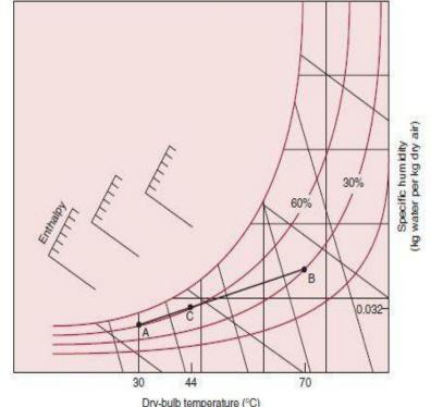
EXAMPLE 9.8: HEATED AIR AT 50C AND RELATIVE HUMIDITY IS USED TO DRY RICE IN A 08% DRYER. THE AIR EXITS THE BIN UNDER SATURATED CONDITIONS. DETERMINE THE AMOUNT OF WATER REMOVED PER KG OF DRY AIR.
