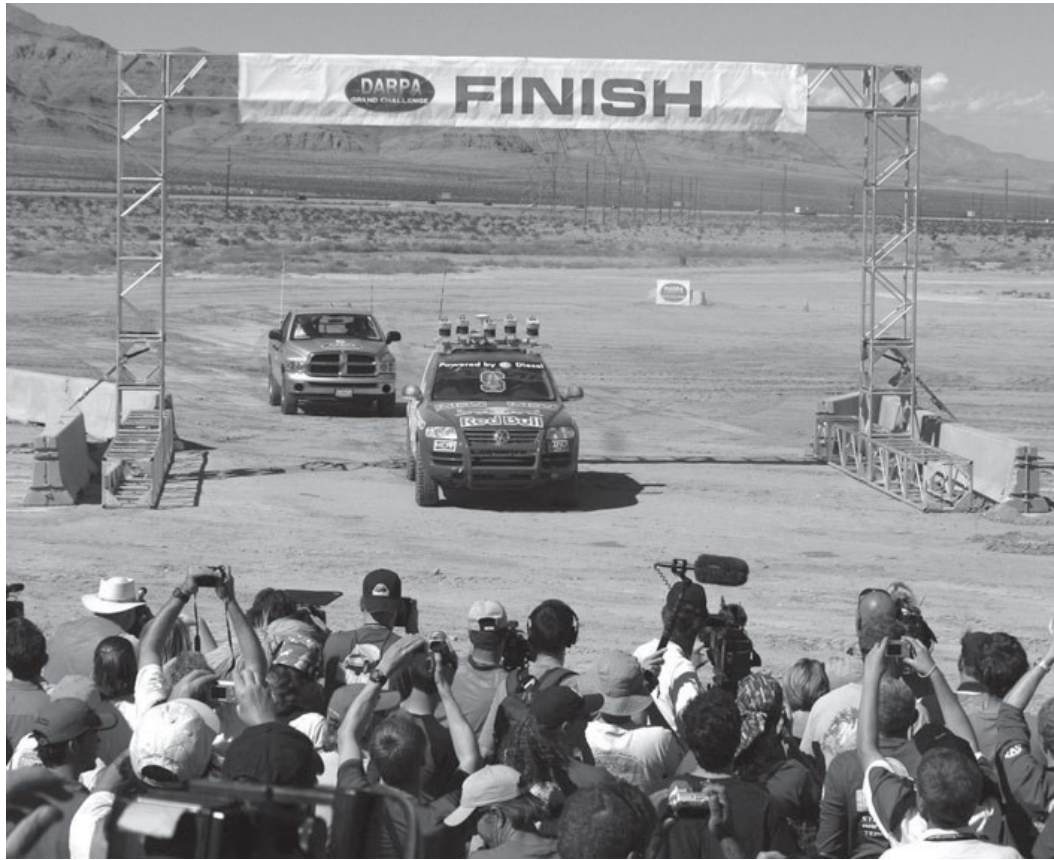
FIGURE 10.4 The Stanford Racing Team converted a Volkswagen Touareg into an autonomous vehicle named Stanley that successfully followed a 128-mile course through the Nevada desert in 2005. (© Gene Blevins/Reuters/Corbis)
