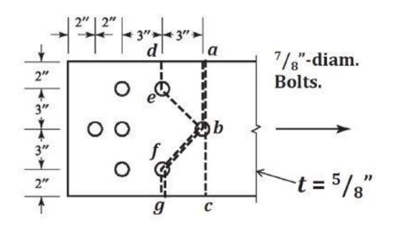
Plate is under tension form one side only. Failure line shall be investigated from loaded side only. Failure line shall be such that intact bolts may not be present on both sides of the failure line.
