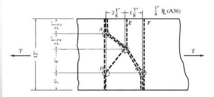
Plate is under tension form both sides. Failure line shall be investigated from both sides. Failure line shall be such that intact bolts may not be present on both sides of the failure line.
