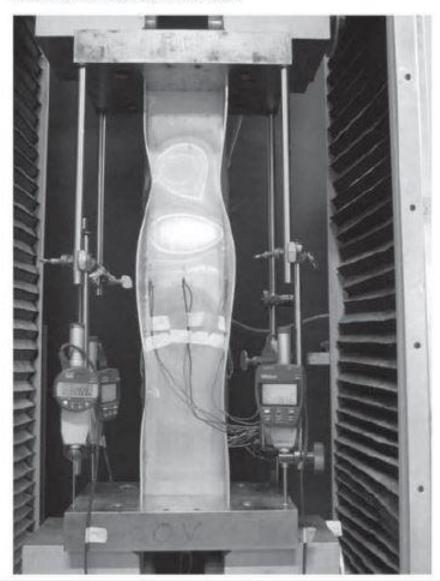
Local buckling primarily depends on the ratio, b/t, of the width (b) and thickness (t) of the plate elements that builds up a section.
