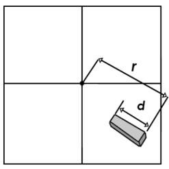
Example: The length of a displaced building is measured at 2.01 mm and the radial distance to the principal point is 56.43 mm. If the the flying height about the surface is 1220 m, what is the height of the building?
