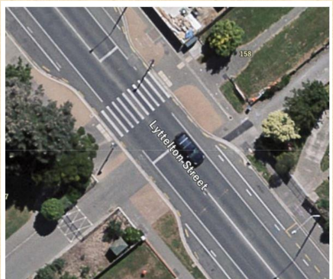
Kerb extensions to support a zebra crossing, Christchurch. (Source: Canterbury maps)
