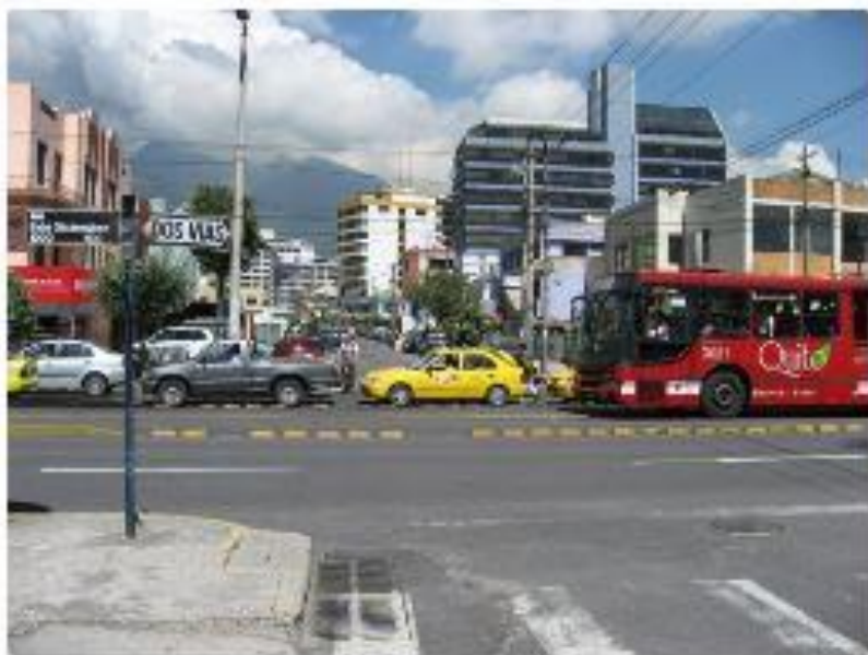
Fig. 24.31 Prior to Quito's Ecovía line, mixed-traffic vehicles were allowed to cross through this intersection as well as negotiate cross-traffic and curbside turns. To give priority to public transport, crossing straight and cross-traffic turn movements have been blocked. Lloyd Wright.
