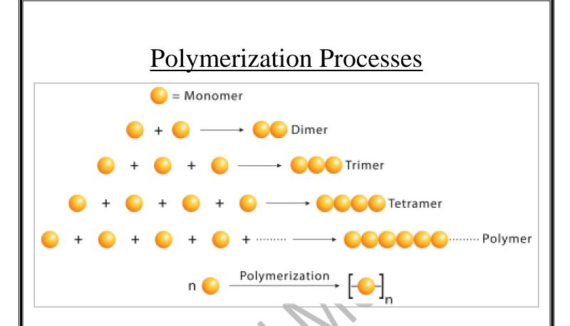
A process of making the **monomer molecules react together** in a chemical reaction and produce three-dimensional networks or **polymer chains** is called **polymerization**.
