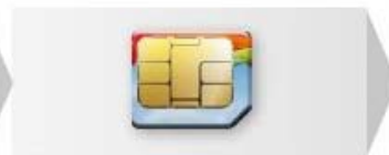
Micro-SIM / 3FF (2004) 15 x 12 mm (180 mm 2 )
