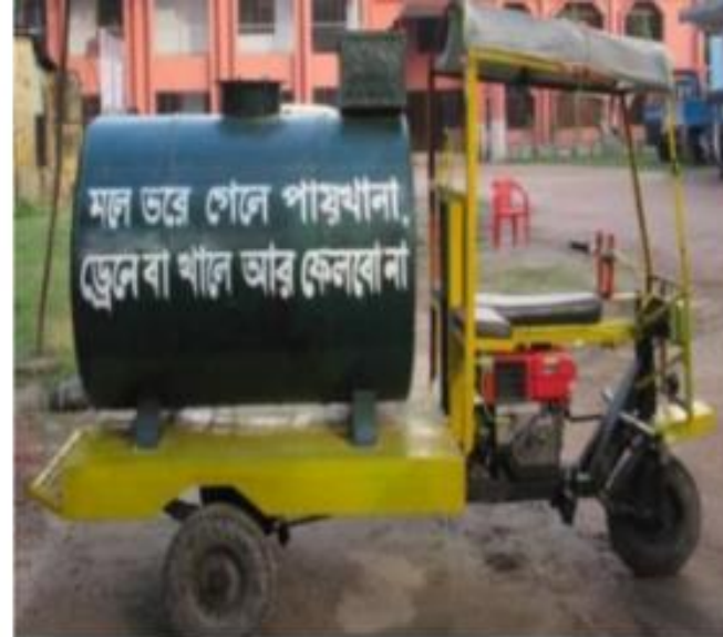
Mechanized Transporter (Mounted on Tri-Wheeler Diesel Engine Driven Vehicle); Capacity: 1000 Liters
