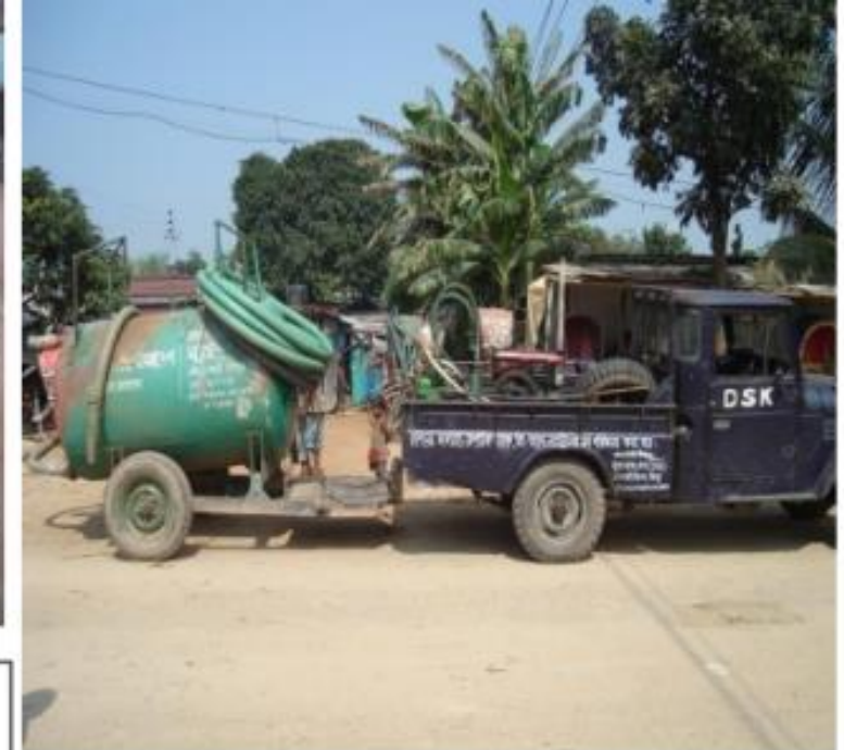
Mechanized transport of fecal sludge
